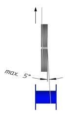
In the case of hollow conductors, in connection with high installation tensile stresses, the brake drum grooves must be adapted to the cable diameter. This is to prevent the hollow conductor becoming permanently deformed in the area of the brake drum cable wrap.
